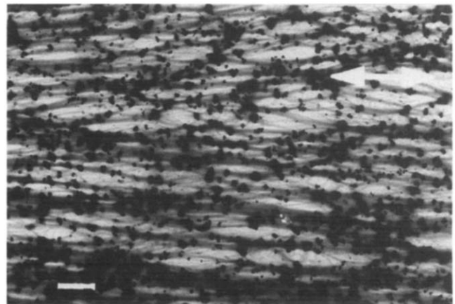
Figure 3 Stretched, carbon-black-filled (40 phr, Corax N 765) sample viewed in the transmission electron microscope. The white bar marks 1100 nm and the arrow indicates the direction of stress
